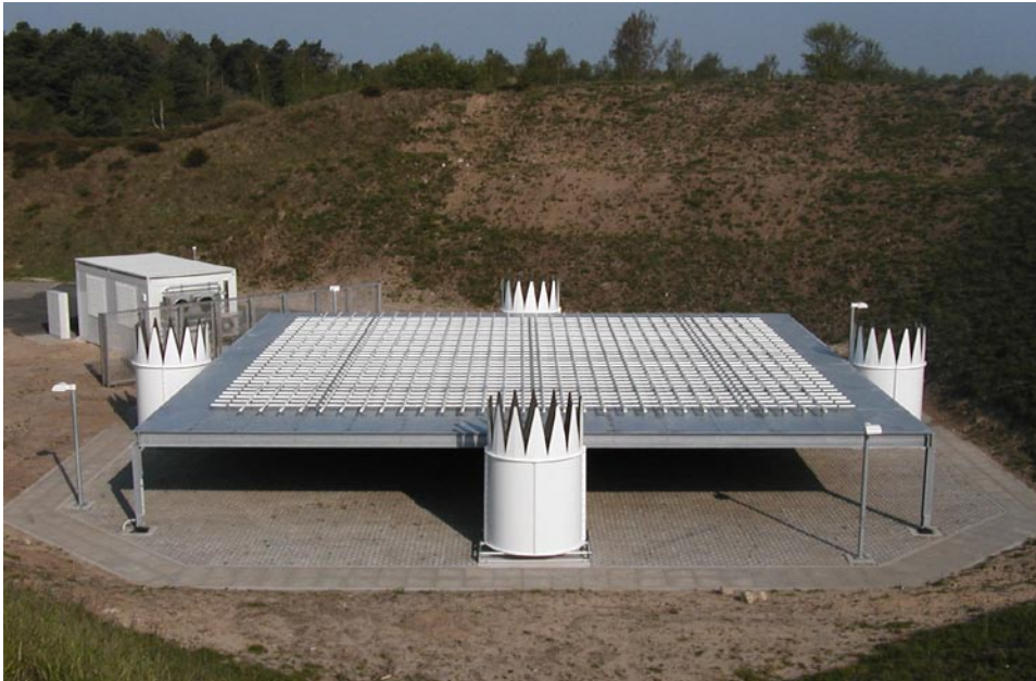
Vaisala LAP ® -16000 with RASS in Germany.
