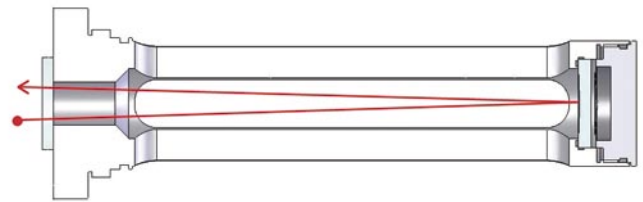
The passage of light in the SPECTRACAP® sensor probe used in the OMT355.
